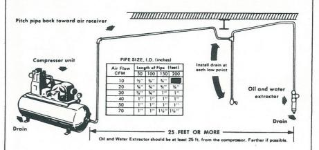
The oil and water extractor should not be mounted on or near the air compressor.
