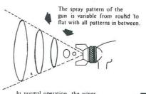
In normal operation, the wings on the nozzle are horizontal as illustrated here. This provides a vertical fan shaped pattern which gives maximum coverage as the gun is moved back and forth parallel to the surface being fin-
