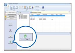
If the software version is older than 1.20, a communication error (protocol error) occurs in any communications attempted between the instrument and Wireless Logger Collector.
